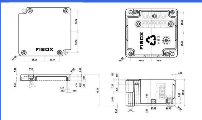
Including: Base, cover with gasket, cover screws and terminal block (4~30pins).
