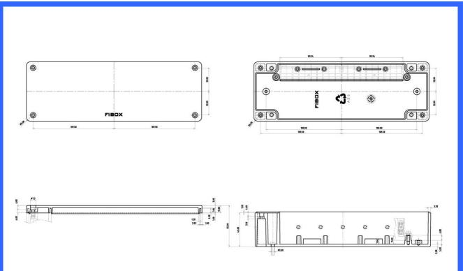
Including: Base, cover with gasket, cover screws and terminal block (4~30pins).
