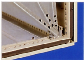
安裝板下端之固定方式，2.3m/m鍍鋅鋼板，周邊均折曲成寬24m/m之C形彎邊，確保配盤作業更為方便，提高安裝板之剛性，且便於搬運。 The mounting plates are 2.3mm galvanized steel plate. All sides of the plates are banded to 24mm wide C-form edge to reinforce the rigidity of the plates. It also makes the transport and cable installation more convenient.
