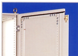
堅固的箱門長方形補強框條上，每相隔25m/m均設有嵌孔，可以固定電線槽、電纜束、線路圖插袋等，箱門如需再開孔加工時，長方形補強框條亦可簡單卸下。 The robust strengthening bars of the enclosure's door has punched hole for every 25mm. The cable grooves, cable bundles and cable drawing bags can be easily put on the enclosure's door. The strengthening bars can be disassembled easily if the door is to rework later, e.g. for hole punching.
