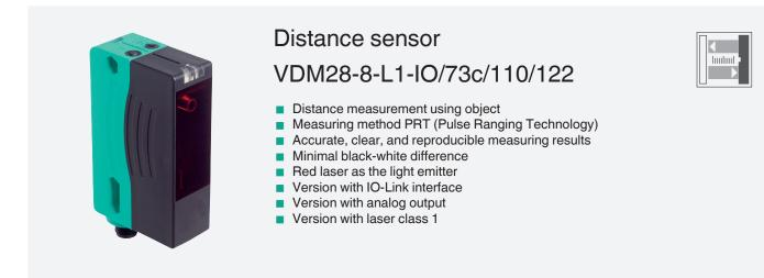
Universal distance sensor, measurement to object, IO-Link interface, measuring method PRT, 8 m detection range, red laser light, laser class 1, push-pull output, analog output, M12 plug
