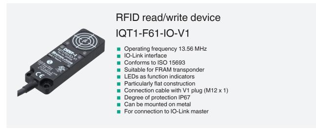
HF RFID read/write device with IO-Link in accordance with ISO 15693
